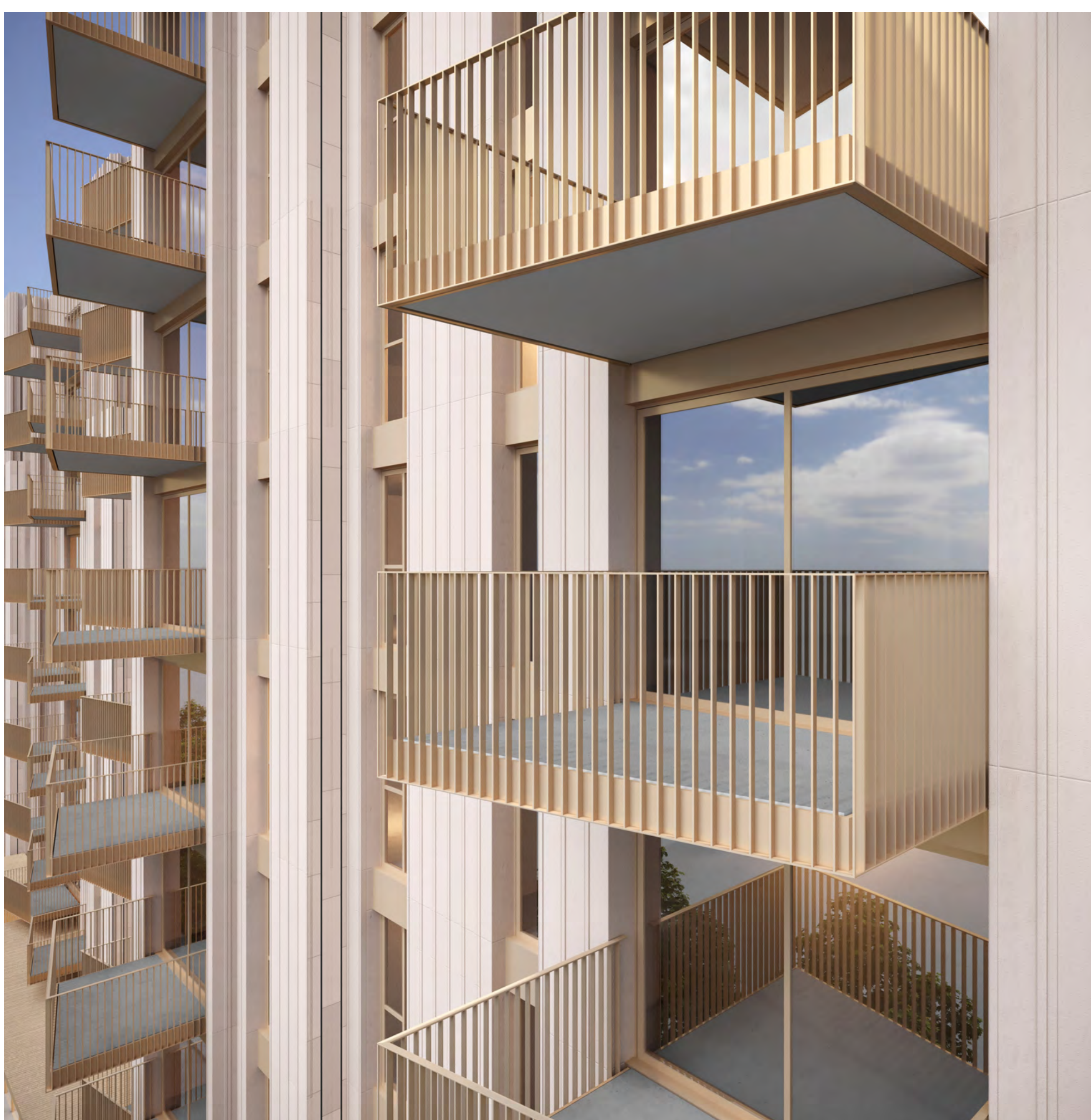
Terracotta cladding. Warm and light yellow/Beige/Buff tone. Portrait panel orientation with vertical jointing will emphasise the verticality. Horizontal joints to be butt jointed to minimise visibility. Simple, elegant, metal balcony balustrades. Light bronze/ Champagne tone.
